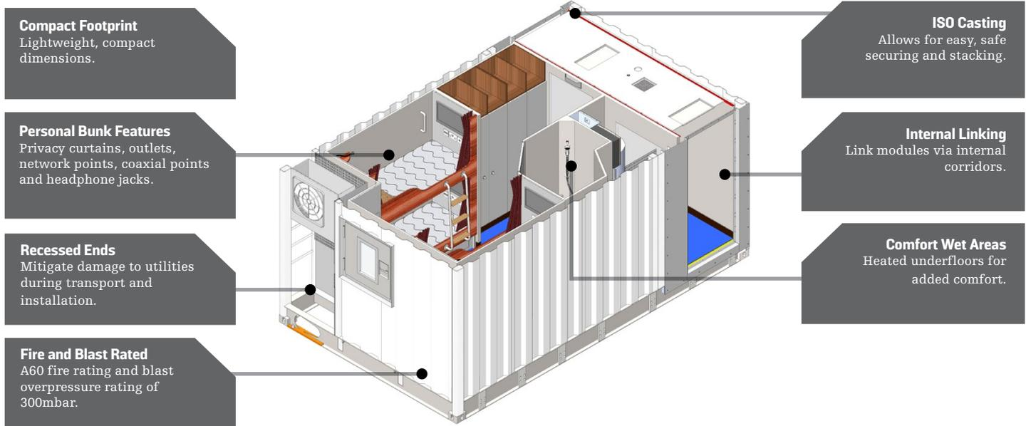
HB Rentals' 18' DNV A60 Linkable Sleeper is designed to accommodate up to 4 individuals. Certified to DNV 2.7-1, the 18' sleeper module can be utilized where heavier, larger modules cannot be. The module provides easy plug and play connections with safe and quick installation features. Superior engineering allow modules to link horizontally and stack up to four units high, depending on the vessel type.
